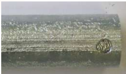
Obr. 13: Strupovitost na trubce
