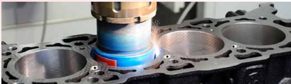
Obr. 3: Gehring, Laser honing [9]
